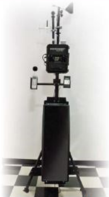
HAZ-SCANNER EPAS shown with optional solar panels
