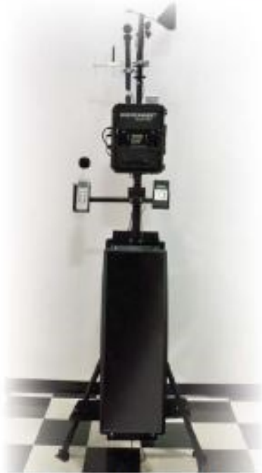
HAZ-SCANNER EPAS shown with optional solar panels
